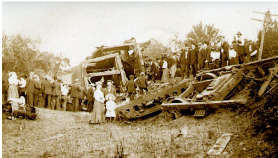
The baggage car was telescoped the whole length of the forward passenger car.
